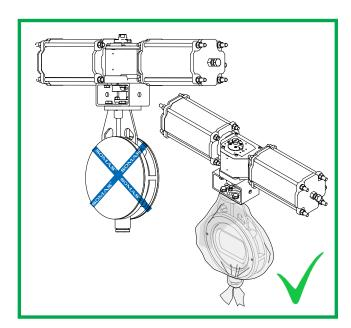
Keep the valve and its accessories in its original packaging during storage.
